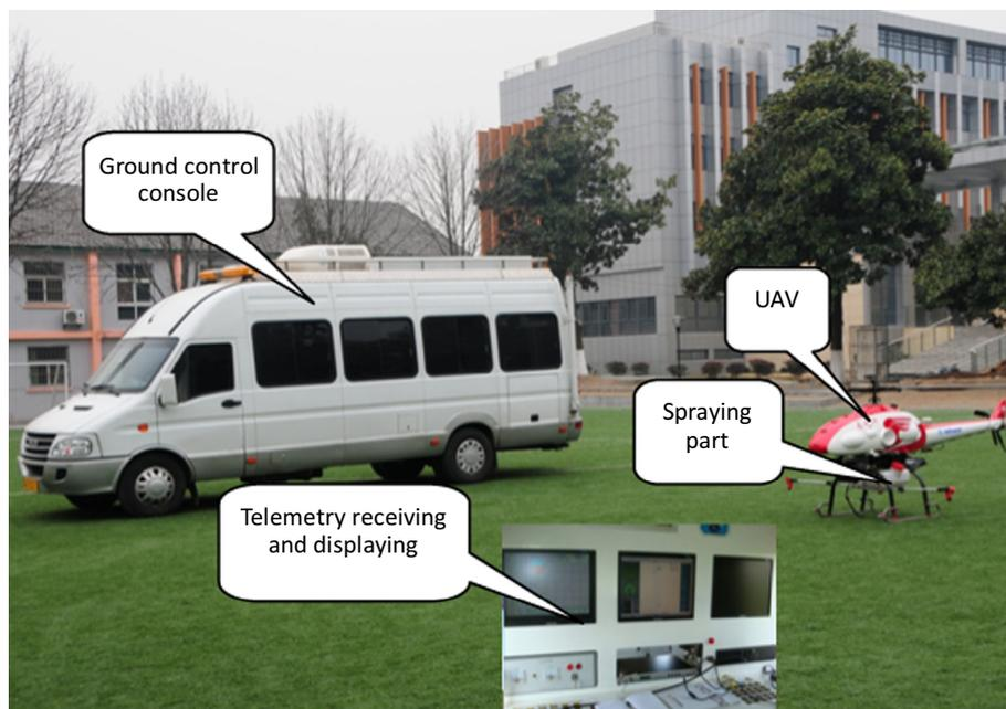
Fig. 1. N-3 type of spraying helicopter system structure diagram.
