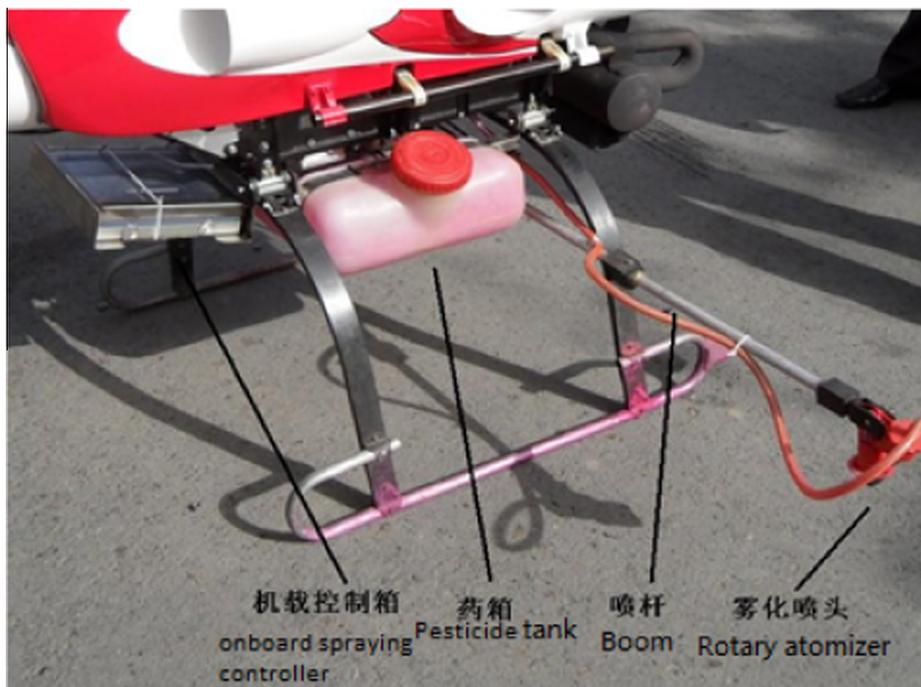
Fig. 5. Onboard spraying system.
