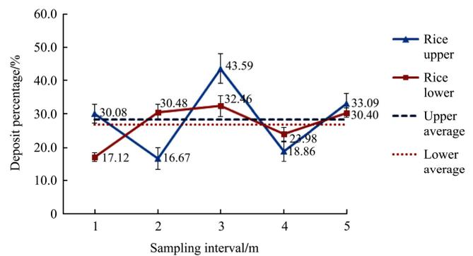
Figure 4 Rice upper and lower deposition (cm<sup>2</sup>)
