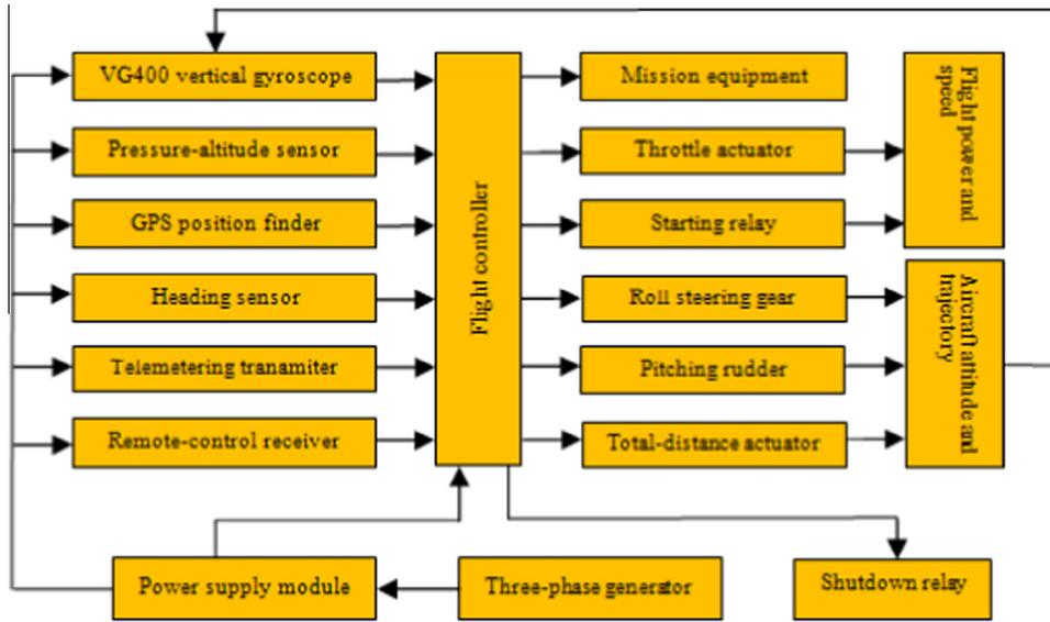
Fig. 2. UAV flight control system chart.
