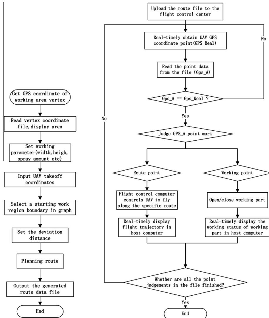
Fig. 6. Control system software flow chart.
