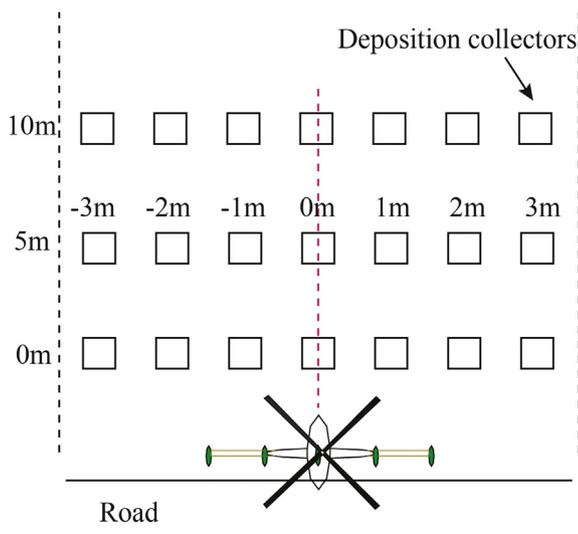
**Fig. 2.** Layout of the droplet sampling cards (top view).
