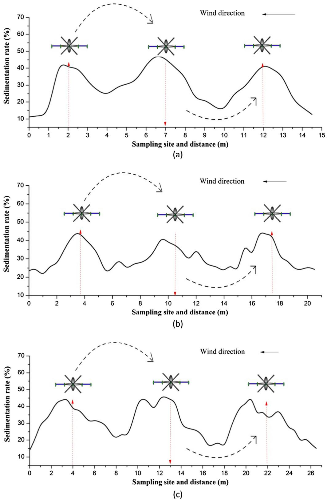
(a) Flight height 5m; spray swath 5m; spray droplet diameter 250µm; (b) Flight height 5m; spray swath 7m; spray droplet diameter 250µm; (c) Flight height 5m; spray swath 9m; spray droplet diameter 250µm
