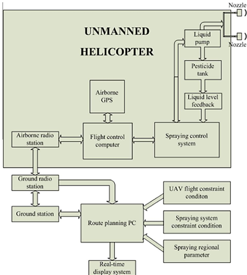
Fig. 3. Spraying control system structure of N-3.
