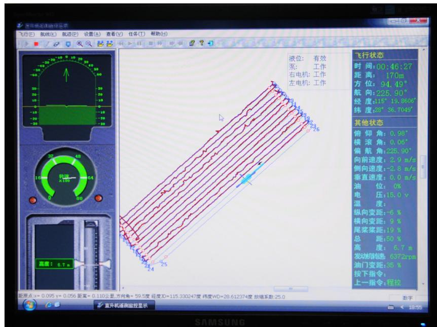
Fig. 7. Real-timely displayed route map in monitoring equipment.
