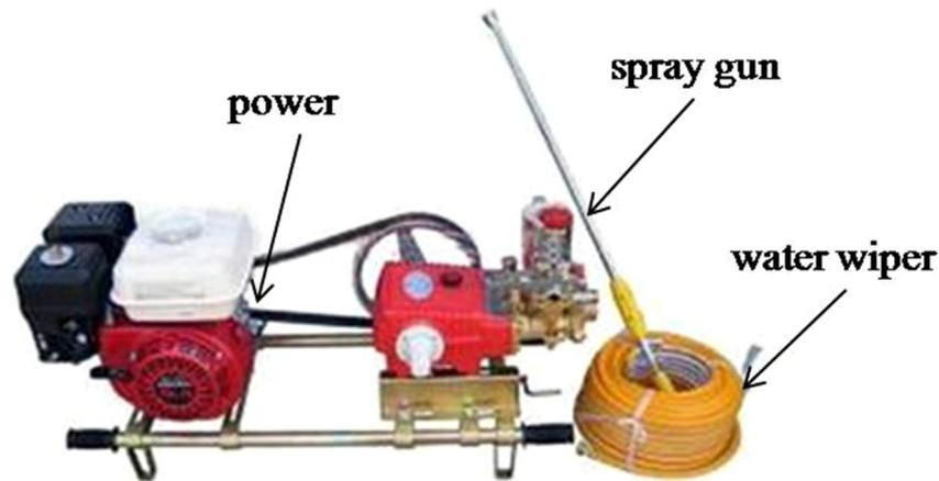
**Fig. 1.** The diagram of stretcher-mounted sprayer.
